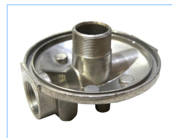
Filter Holder Item. No. TSFS-GL-5 Material: aluminum In/outlet: 1" Size: 1 1/2"-16UNF
